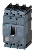
circuit breaker 3VA5 UL frame 125 3-pole, starter protection TM120M, AM, In=125A without overload protection short-circuit protection li=3...7 x In nut keeper kit on both sides
