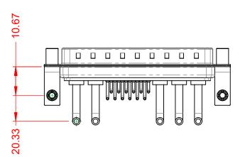
POWER/CO-AX CONTACT RATING:20A (CURRENT)(IF PRESENT)SIGNAL CONTACT CURRENT RATING:5A PER CONTACTSIGNAL CONTACT RESISTANCE:10mΩ MAX.INSULATOR RESISTANCE:5000MΩ min.DIELECTRIC5000MΩ min.
