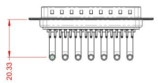
30A (CURRENT) POWER/CO-AX CONTACT RATING: (IF PRESENT) SIGNAL CONTACT CURRENT RATING: 5A PER CONTACT SIGNAL CONTACT RESISTANCE:  $10m\Omega$  MAX. INSULATOR RESISTANCE: 5000MΩ min. DIELECTRIC
