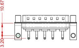
10A (CURRENT) POWER/CO-AX CONTACT RATING: (IF PRESENT) SIGNAL CONTACT CURRENT RATING: 5A PER CONTACT SIGNAL CONTACT RESISTANCE:  $10m\Omega$  MAX.
