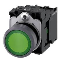
Illuminated pushbutton, 22 mm, round, plastic with metal front ring, green, pushbutton, flat, momentary contact type, with holder, 1NO, LED module with integrated LED 110 V AC, screw terminal, with laser labeling, lower case
