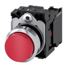
Pushbutton, 22 mm, round, metal, shiny, red, pushbutton, raised, momentary contact type, with holder, 1 NC, screw terminal, with laser labeling, lower case
