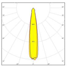
Dimensions: 49.9 mm x 49.9 mm Height: 24.00 mm ~15° spot beam
