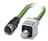
Network cable, PROFINET CAT5 (100 Mbps), EtherCAT® CAT5 (100 Mbps), 4-position, PVC/PVC, green RAL 6018, shielded, Plug straight RJ45 Push Pull / IP67, on Socket straight M12 SPEEDCON / IP67, coding: D, cable length: 2 m
