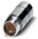
Coupler connector, straight, Screw locking, M23, number of positions: 12, type of contact: Pin, Crimp connection, shielded: yes, cable diameter range: 9 mm ... 13.2 mm
