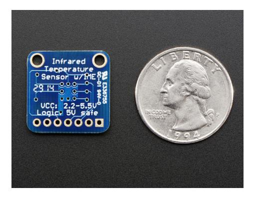
Simply point the sensor towards what you want to measure and it will detect the temperature by absorbing IR waves emitted. The embedded thermopile sensor generates a very very small voltage depending on how much IR there is, and using some math, that micro voltage can be used to calculate the temperature. It also takes the measurement over an area so it can be handy for determining the average temperature of something.
