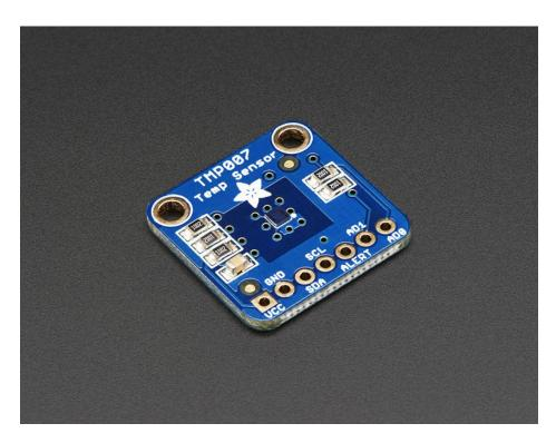
Unlike most of the other temperature sensors we have, this breakout has a really cool IR sensor from TI that can measure the temperature of an object without touching it.
