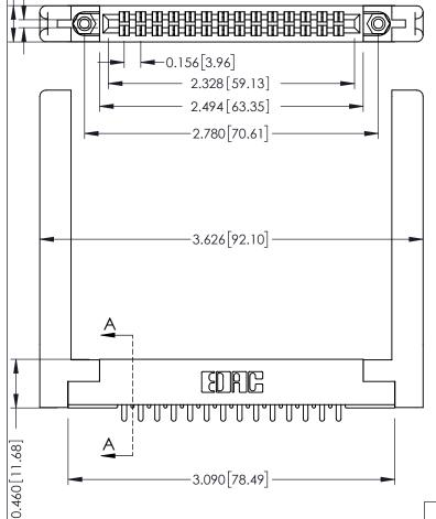
0.295[7.49] Card Slot SECTION 0.090[2.29] Point of Contact 305 ENG MASTER 305 / 315 / 355 Card Edge Connector
