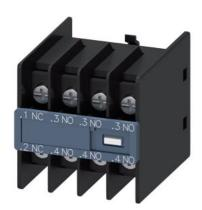
Auxiliary switch on the front, 3 NO + 1 NC Current path 1 NC, 1 NO, 1 NO, 1 NO for 3RH and 3RT Ring cable lug connection .1/.2, .3/.4, .3/.4, .3/.4
