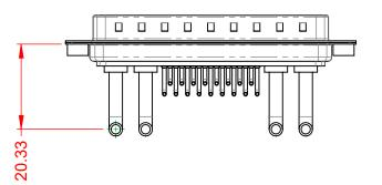
POWER/CO-AX CONTACT RATING:30A (CURRENT)(IF PRESENT)SIGNAL CONTACT CURRENT RATING:5A PER CONTACTSIGNAL CONTACT RESISTANCE: $10m\Omega$  MAX.INSULATOR RESISTANCE:5000MΩ min.DIELECTRICDIELECTRIC
