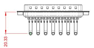
POWER/CO-AX CONTACT RATING:20A (CURRENT)(IF PRESENT)SIGNAL CONTACT CURRENT RATING:5A PER CONTACTSIGNAL CONTACT RESISTANCE: $10m\Omega$  MAX.INSULATOR RESISTANCE:5000MΩ min.DIELECTRICDIELECTRIC
