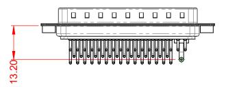
10A (CURRENT) POWER/CO-AX CONTACT RATING: (IF PRESENT) SIGNAL CONTACT CURRENT RATING: 5A PER CONTACT SIGNAL CONTACT RESISTANCE:  $10m\Omega$  MAX. **INSULATOR RESISTANCE:** 5000MΩ min.
