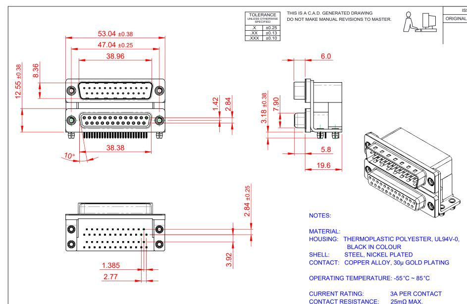
WITHSTANDING VOLTAGE: 1000V AC rms
