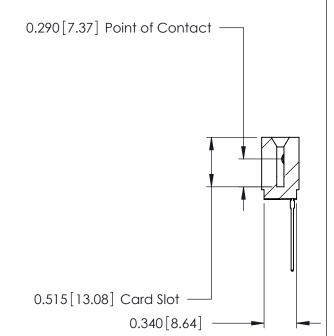
746 Series Ultra-Mate Card Edge Connector - Press Fit
