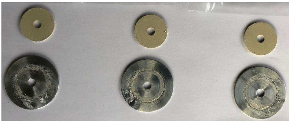
Aluminium 6061-T6 coupons and their associated Silicone Silver Aluminium gaskets after 504 hours of salt-fog exposure.
