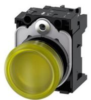
Indicator lights, 22 mm, round, plastic, yellow, lens, smooth, with holder, LED module, with integrated LED 24 V AC/DC, screw terminal, with laser labeling, lower case
