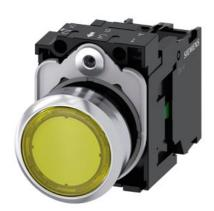
Illuminated pushbutton, 22 mm, round, metal, shiny, yellow, pushbutton, flat, momentary contact type, with holder, 1NO, LED module with integrated LED 24 V AC/DC, screw terminal, with laser labeling, symbol number according to, ISO 7000 or IEC 60417
