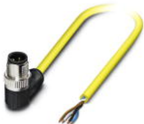
Sensor/actuator cable, 4-position, PVC, yellow, Plug angled M12 SPEEDCON, A-coded, on free cable end, cable length: 2 m
