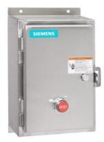
Non-reversing motor starter, Size 0, Three phase full voltage, Solid-state overload relay, OLR amp range 0.75-3.4A, 24VAC 50-60Hz coil, Non-combination type, Encl. type 4X 304 S. Steel, Water/dust tight noncorrosive, Standard width enclosure
