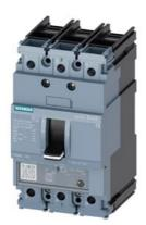
circuit breaker 3VA5 UL frame 125 breaking capacity class M 35kA @ 480 V 3-pole, line protection TM230, FTAM, In=50A overload protection Ir=50A fixed short-circuit protection Ii=5...10 x In UL489 SB (naval), 50 deg. cel. cable connection on both sides
