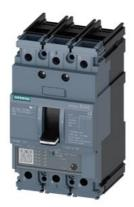
circuit breaker 3VA5 UL frame 125 3-pole, starter protection TM120M, AM, In=15A without overload protection short-circuit protection li=5...12 x In nut keeper kit on both sides
