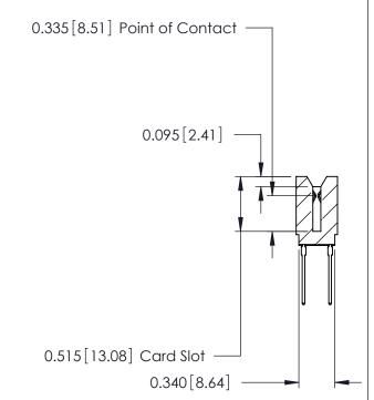
746 Series Ultra-Mate Card Edge Connector - Press Fit Part Number: 746-060-545-206
