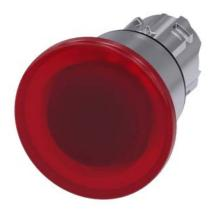
Illuminated mushroom pushbutton, 22 mm, round, metal, shiny, red, 40mm, latching, pull-to-unlatch mechanism, with laser labeling, inscription or symbol Customer-specific selection with SIRIUS ACT configurator (CIN)
