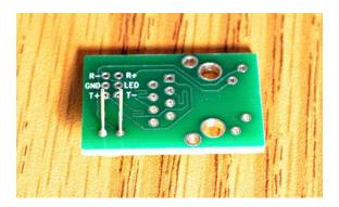
Next solder the header pins. After soldering 1 pin, turn the board over to check if the pins are at a right angle to the board. Once 2 or more pins are soldered, fixing crooked pins is almost impossible.
