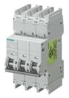
Miniature circuit breaker 240 V 14kA, 3-pole, D, 10A, D=70 mm according to UL 489  $\,$
