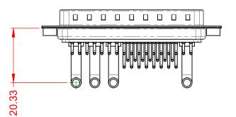
40A (CURRENT) POWER/CO-AX CONTACT RATING: (IF PRESENT) SIGNAL CONTACT CURRENT RATING: 5A PER CONTACT SIGNAL CONTACT RESISTANCE:  $10m\Omega$  MAX. **INSULATOR RESISTANCE:** 5000MΩ min.
