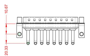
OPERATING TEMPERATURE: $-55^{\circ}C \sim 125^{\circ}C$ POWER/CO-AX CONTACT RATING:20A (CURRENT)(IF PRESENT)SIGNAL CONTACT CURRENT RATING:5A PER CONTACTSIGNAL CONTACT RESISTANCE:10m $\Omega$  MAX.INSULATOR RESISTANCE:5000M $\Omega$  min.DIELECTRIC2000M $\Omega$  min.
