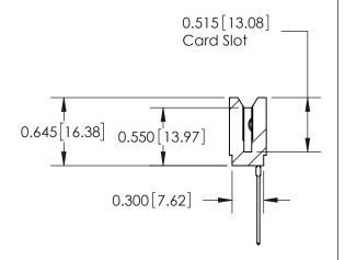
ACAD REFERENCE NO. 737 Series Ultra-Mate Card Edge Connector - Press Fit DRAWN: Part Number: 737-012-541-106 CHECKED: **EDAC INC** SCALE: THESE DRAWINGS AND SPECIFICATIONS ARE THE PROPERTY OF EDAC INC.,AND TORONTO, ONTARIO SHALL NOT BE REPRODUCED, OR COPIED DRAWING NUMBER CANADA OR USED AS THE BASIS FOR THE MANUFACTURE OR SALE OF APPARATUS YOUR CONNECTION TO QUALITY & SERVICE WITHOUT WRITTEN PERMISSION.
