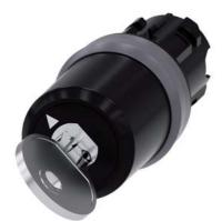
Key-operated switch BKS, 22 mm, round, plastic with metal front ring, special lock, with 2 keys, 2 switch positions O<I, momentary contact type, actuating angle 45°, 10:30h/12h, key removal O, Note: BKS locking systems E1 - E25 supplied without key
