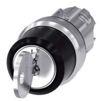
RONIS key-operated switch, 22 mm, round, metal, shiny, lock number SB30, with 2 keys, 3 switch positions I-O-II, latching, actuating angle 2x45°, 10:30h/12h/13:30h, key removal O+I, possible special locks: SB31, 421, 455, with laser labeling, upper case and lower case, always upper case at the beginning of the word
