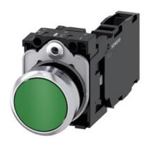
Pushbutton, 22 mm, round, metal, shiny, green, pushbutton, flat, momentary contact type, 1 NO+1 NC, screw terminal, with laser labeling, symbol number according to, ISO 7000 or IEC 60417
