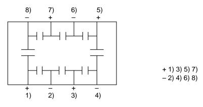
8 terminals are connected and measured at the same time.
