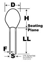
**General Information** Series T350 Dielectric MnO2 Tantalum Style Radial Description Radial, Solid Tantalum, Conformal, Dipped Features Low Leakage RoHS No MARNING: Cancer and reproductive harm -Prop 65 http://www.p65warnings.ca.gov. SCIP 0c1392c3-c7b9-4178-827c-fa26617a3178 Number Termination Lead (SnPb) AEC-Q200 No Notes Longest Lead Is Positive.
