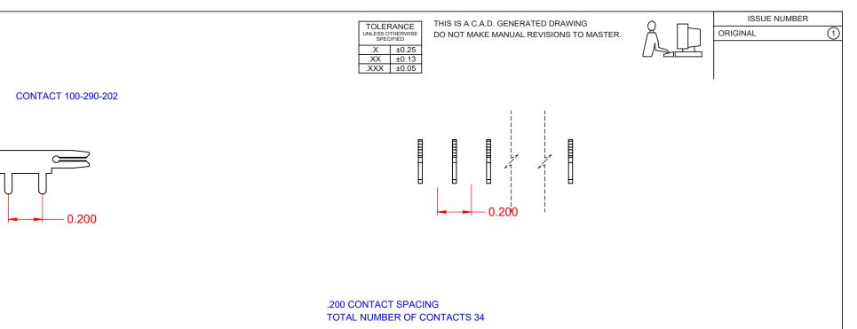
NOTE: CONTACTS ARE HELD IN A CARRIER FOR EASE OF ASSEMBLY
