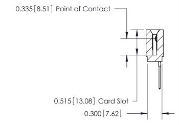
ACAD REFERENCE NO. 745 Series Ultra-Mate Card Edge Connector - Press Fit DRAWN: J.LEE Part Number: 745-040-545-101 CHECKED: **EDAC INC** SCALE: THESE DRAWINGS AND SPECIFICATIONS ARE THE PROPERTY OF EDAC INC., AND TORONTO, ONTARIO SHALL NOT BE REPRODUCED, OR COPIED DRAWING NUMBER CANADA OR USED AS THE BASIS FOR THE 745-ENG MASTER MANUFACTURE OR SALE OF APPARATUS YOUR CONNECTION TO QUALITY & SERVICE WITHOUT WRITTEN PERMISSION.
