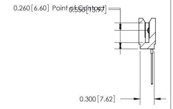
745 Series Ultra-Mate Card Edge Connector - Press Fit Part Number: 745-045-541-106
