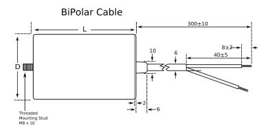
Series C27 Dielectric Film/Foil Polypropylene Style Plastic Case and Cover, Ultra Sonically Welded Description Ultra Sonically Welded Seal, Safety Class PO, **Features** UL 94 V0 Disk RoHS Yes Termination Tin Copper Lead BiPolar Cables UL, VDE, UL (Construction Only), UL\_94 VO Disk Qualifications AEC-Q200 Component 77.85 q Weight
