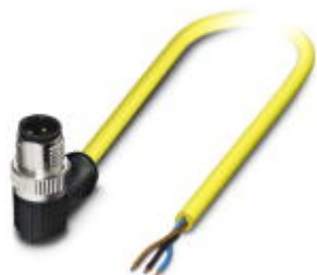
Sensor/actuator cable, 3-position, PVC, yellow, Plug angled M12 SPEEDCON, A-coded, on free cable end, cable length: 2 m
