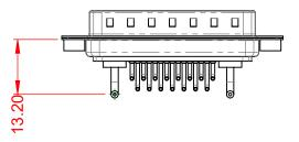
10A (CURRENT) **POWER/CO-AX CONTACT RATING:** (IF PRESENT) SIGNAL CONTACT CURRENT RATING: 5A PER CONTACT SIGNAL CONTACT RESISTANCE:  $10m\Omega$  MAX. INSULATOR RESISTANCE: 5000MΩ min.
