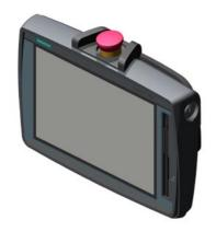
SIMATIC HMI TP1000F MOBILE 10.0" TFT display, 1280x800 pixels, 16 million colors, Touch operation, touch pen, 1x PROFINET/Industrial Ethernet interface, 1x multimedia card, 1x USB, key-operated switch, acknowledgement button, 1 emergency stop/stop button confligurable from WinCC Comfort V14
