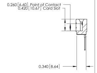
726 Series Ultra-Mate Card Edge Connector - Press Fit Part Number: 726-009-540-101 **EDAC INC** THESE DRAWINGS AND SPECIFICATIONS ARE THE PROPERTY OF EDAC INC.,AND TORONTO, ONTARIO SHALL NOT BE REPRODUCED, OR COPIED CANADA OR USED AS THE BASIS FOR THE MANUFACTURE OR SALE OF APPARATUS YOUR CONNECTION TO QUALITY & SERVICE
