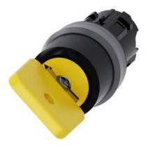
Key-operated switch O.M.R, 22 mm, round, plastic with metal front ring, lock number 73033, yellow, with 2 keys, 2 switch positions O<I, momentary contact type, Actuating angle 45°, 10:30h/12h, key removal O, Z=50-unit packaging
