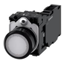
Illuminated pushbutton, 22 mm, round, plastic, white, pushbutton, flat, momentary contact type, with holder, 1 NO+1 NC, LED module with integrated LED 110 V AC, screw terminal, Z=20-unit packaging
