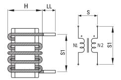
General InformationSeriesSC-DStyleThrough-HoleRoHSYesNotesLead Spacing (S/S1) Are For Reference Only.MiscellaneousTemperature Rise Maximum: 45 K.CoreNi-Zn Ferrite
