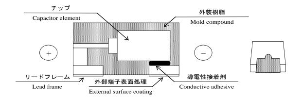
Lead frame base : Iron-Nickel alloy/Copper plating
