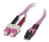
Assembled FO cable, zip cord cable, multi-mode fiberglass 50/125  $\mu$ m, OM4, plug: LC/SC duplex, degree of protection: IP20, for installation in cable ducts or control cabinets, length: 1 m
