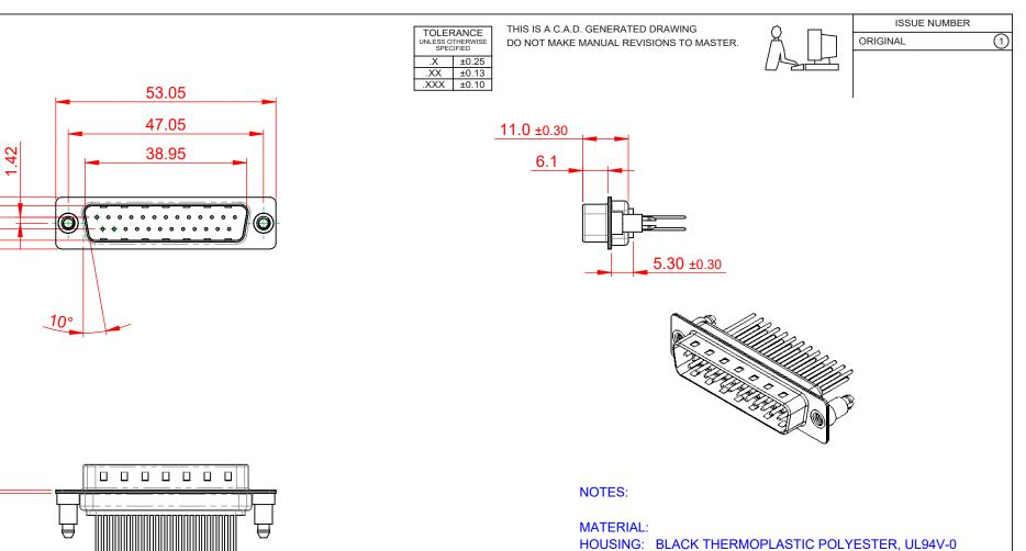
STEEL, NICKEL PLATED SHELL: CONTACT: COPPER ALLOY, GOLD FLASH PLATED
